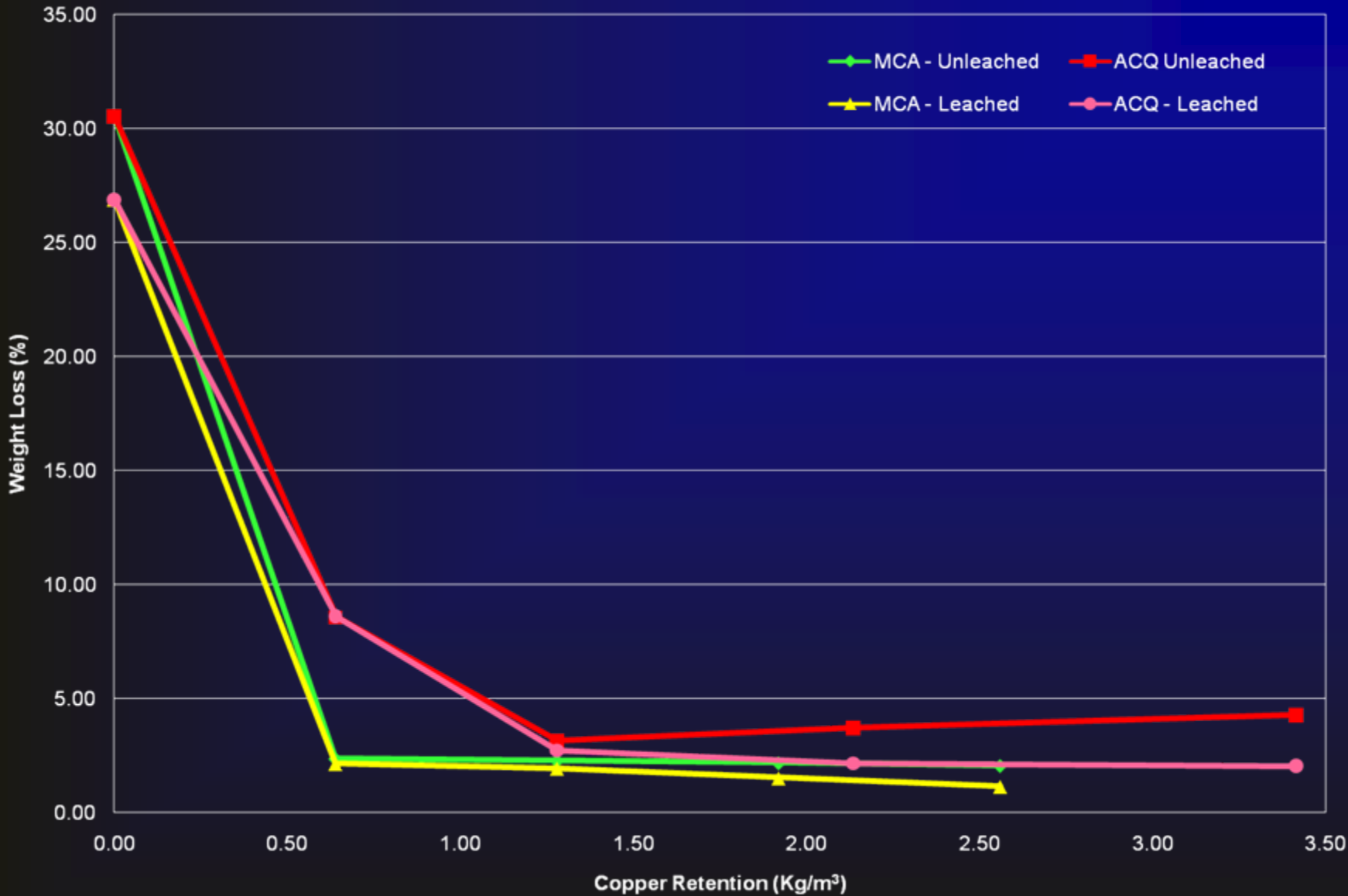
Weight Loss of MCA and ACQ-Type D Treated Southern Pine Soil Blocks after an 8-Week AWP A E10-06 Exposure to Gloeophyllum trabeum
